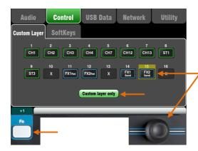
The Custom layer can have any combination of channel, FX and master strips assigned to its faders.
