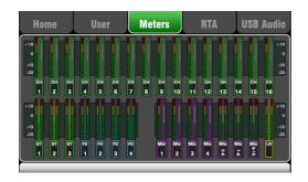
This screen provides a convenient view of all channel, mix and FX signal activity.
