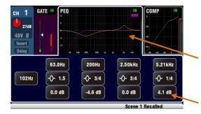
**Processing Screen** – When selected this screen presents the processing such as Preamp, EQ, Gate, Compressor for the channel or master currently selected using its strip **Sel** key.
