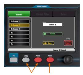
**To Clear a Scene** – Press and hold down the Reset key below the screen and then touch the scene in the list. This clears the scene contents and name.
