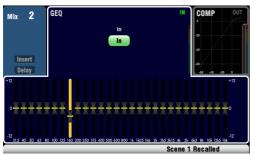
Press the **GEQ Fader Flip** key to view and adjust the GEQ on the faders while a mono or the LR mix is selected. The screen highlights the active range of frequencies. Press the switch again to change range or return to normal mix mode.
