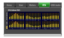
This screen displays a Real Time Analyser (RTA) which analyses the frequency content of the audio signal currently being monitored using the PAFL keys.
