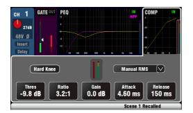
**Frequency** – Each band can sweep its centre point frequency across the full range from 20Hz to 20kHz. This means you can overlap bands and have more precise control over problem frequency areas.
