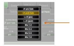
Patch the source to be recorded using the Setup / Audio / Output Patch screen Qu-Drive option menu. The record meter on the USB page displays the current source. The default is LR post-fade.
