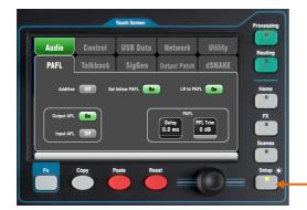
Touch the top tabs to access the different categories of setup function. Touch the tabs below to open up the related options available.
