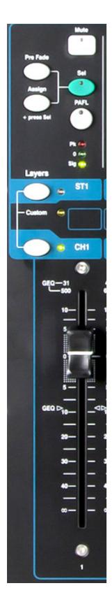
**Mute key** – Press to turn off the channel audio signal. This affects the send to all mixes including LR, effects and stage monitors. The Mute key lights red when the channel is muted. It flashes when it is muted by a Mute Group master.
