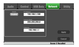
Use this screen set the TCP/IP address for the Network port. It is important that this address is compatible with the addresses of equipment connected to the port, for example a laptop providing MIDI control of mixer parameters, or a wireless router providing remote control using the Qu-Pad iPad app.
