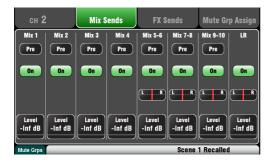
**Routing Screen** – When selected this screen lets you access the assignment and routing for the channel or master currently selected using its strip **Sel** key.
