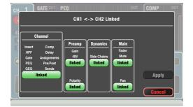
**Linking** lets you gang the preamp, processing and routing of an odd/even mono channel pair for stereo operation. All parameters including the preamp, processing and routing are linked. Pan becomes a width control when linked. Some parameters can be removed from the link using the buttons:
