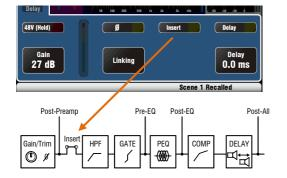
**Delay** up to 85ms can be added to each input channel. In most cases delay is not needed, but can be useful in time aligning sound from the PA to the acoustic sound from an instrument on stage. Allow 1ms per foot distance as a starting point.
