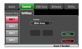
Qu features 4 SoftKeys. These are called 'Soft' because they can be assigned to different functions by the user.
