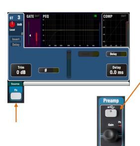
Patch the playback to the ST3 channel using the Processing / Preamp screen Fn key to open the Preamp Source screen. Make sure Qu-Drive is selected as the 'Global USB Source'. Select USB as the source for ST3.
