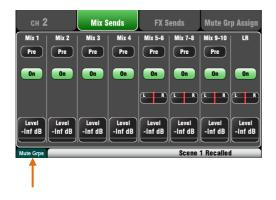
**Function Key** – The **Fn** key provides access to further options associated with the currently selected screen. If available, its function will appear in the lower toolbar above the key. Press the key again to close the option screen.
