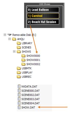
Qu mixer settings can be stored to a USB device (key or drive) plugged into the Qu-Drive port. Data can be archived to computer and transferred between Qu mixers
