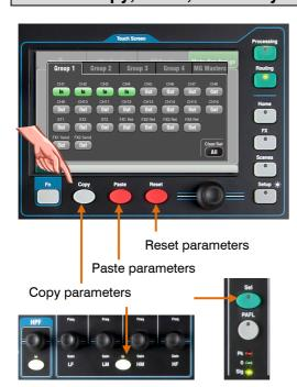
Press + hold down one of these keys and then press another key or screen item to copy, paste or reset the related parameters. For example:
