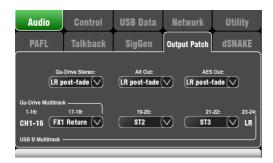
Use this screen to patch signals to the outputs. Touch a box to open up the list of available options. Changes are applied instantly.
