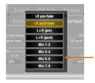
**Button** – Touch to select its function or change its state. To avoid accidental operation some functions need be touched for at least 1 second, for example switching phantom power. These are marked '(Hold)'.
