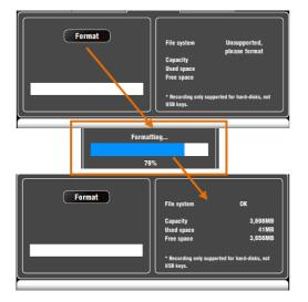
This screen lets you check and format a USB device (key or hard drive) for use with Qu-Drive. Once formatted you do not need to format it again.
